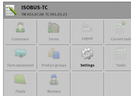
Operating mode: Extended; the "taskdata" folder is not on the SD card.
