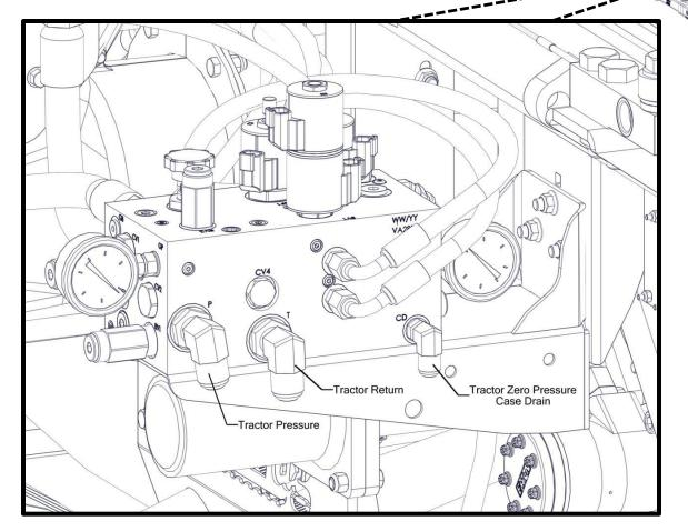
Install hoses in A000177 from tractor to corresponding ports shown.
