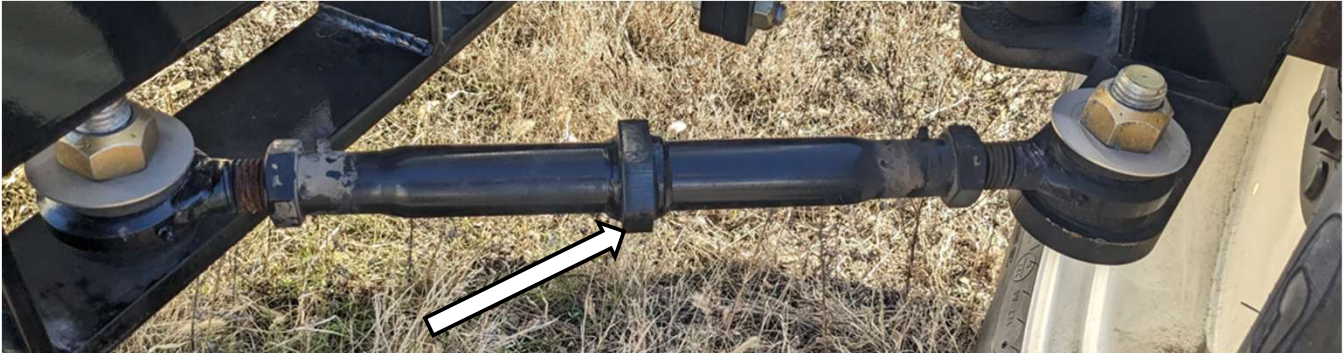
Figure 1: Heavy-duty (current) tie-rod design. Note hex nut on shaft to differentiate from lighter-duty design.
