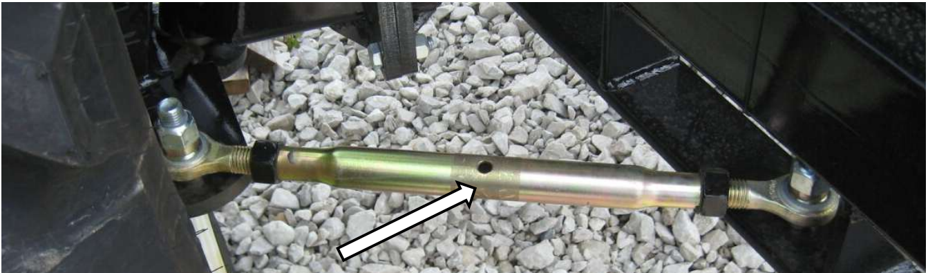
Figure 2: Old tie-rod design. If your tie-rod looks like this, Montag recommends replacing with HD design.
