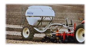
185 CuFt (6 Ton) GEN 1 Base Unit with a white bin on a Montag Auto-Steer Cart shown above. Other color options include gray and yellow (see image below). Bins have two fill inlets. All units use the Montag GEN 1 particulate metering technology.
