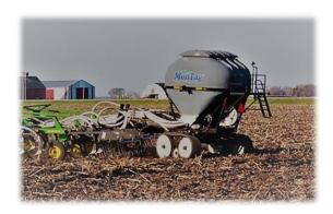
9 Ton GEN 1 Base Unit with a gray bin on a Montag Auto-Steer Cart shown above. Other color options include white and yellow (see image below). Bins have two fill inlets. All units use the Montag GEN 1 particulate metering technology.
