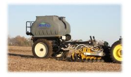
GEN 2 Base Unit with gray bins on a Montag Auto-Steer Cart shown above. Other color options include white and yellow. Bins have two fill inlets each and are independently scaled. All units use the Montag particulate metering system. Multiple U.S. and international patents cover either, or both, this Product and its components.
