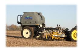
GEN 2 Base Unit with gray bins on a Montag Auto-Steer Cart shown above. Other color options include white and yellow. Bins have two fill inlets each and are independently scaled. All units use the Montag particulate metering system. Multiple U.S. and international patents cover either, or both, this Product and its components.
