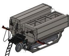
The latest in the GEN 2 product family, the 2224 is designed for operators that need a highly functional and accurate metering system, that also has a carrying capacity of up to 550cu ft or 16 ton of fertilizer.
