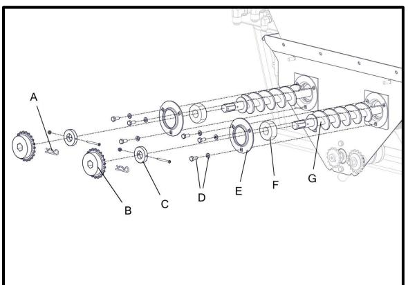
REMOVE PINS (A) FROM END OF AUGER. REMOVE SPROCKETS (B), COLLARS (W/HARDWARE) (C), BEARING FLANGE HARDWARE (D), BEARING FLANGES (E), AND BEARINGS (F). REMOVE EXISTING FULL LENGTH AUGERS (G) FROM METER.
