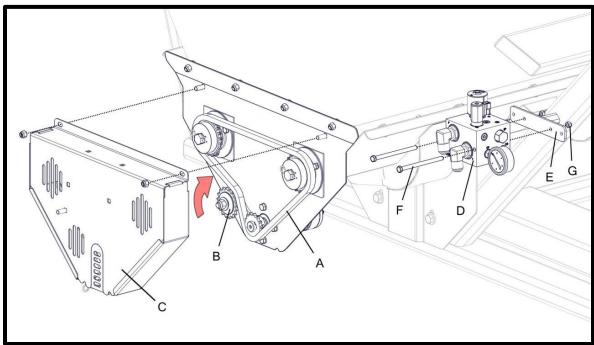
PLACE CHAIN (A) ON SPROCKETS. PUSH TENSIONER (B) UP AGAINST CHAIN TO REMOVE MOST OF THE SLACK, AND FULLY TIGHTEN. CHECK SPROCKET ALIGNMENT. SHIM TENSIONER IF NEEDED. REPLACE COVER (C).
