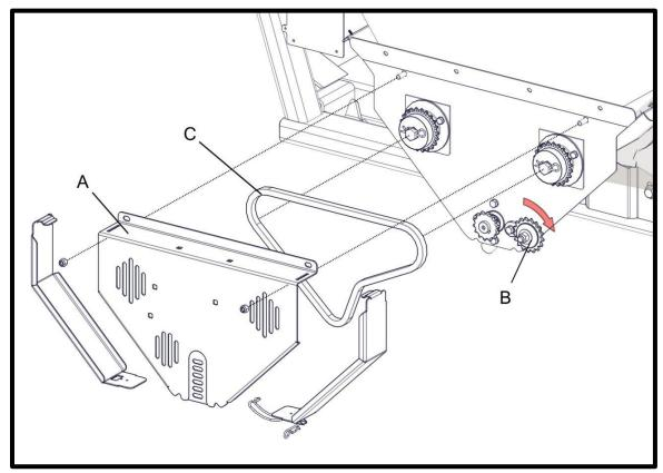
REMOVE COVER (A). LOOSEN CHAIN TENSIONER (B). REMOVE CHAIN (C).
