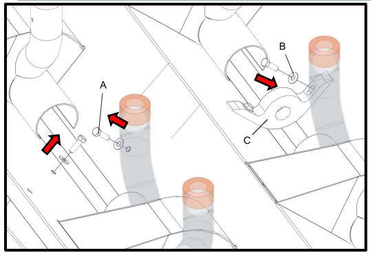
REMOVE BOLTS (A) AND WASHERS (B) FROM CENTER OF METER.
