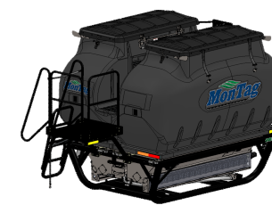
Montag GEN 2 2218 Capacity: 9 Tons Products: 2 Meter Outputs: 1-18 Sections: 1-4 Price: $$$$
