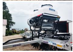
Row Configurable: 2-8 rows Section Configurable: 1-4 sections Slidegate Control Configurable: Manual Lever or Hydraulic Control Bin Size Configurable: 30 ft<sup>3</sup> or 50 ft<sup>3</sup>
