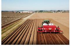
Row Configurable: 2-8 rows Section Configurable: 1-4 sections Slide gate Control: Manual Lever Bin Size Configurable: 30 ft<sup>3</sup> or 50 ft<sup>3</sup>
