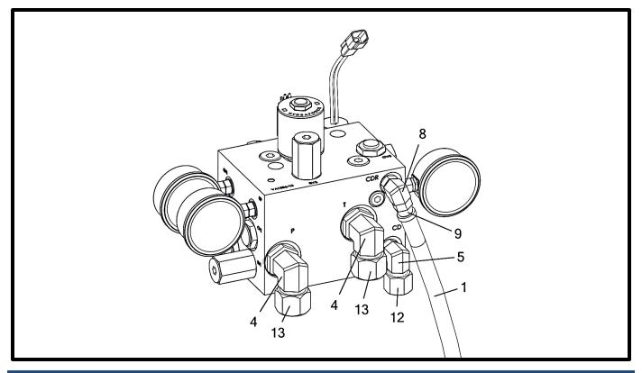
Hydraulic Block - 1 Product Mechanical Slide Gate - Rear View
