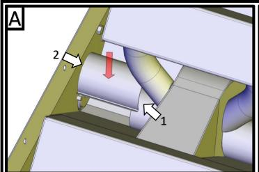
APPLY SILICONE TO TOP OF AUGER COVER (ARROW 1).
