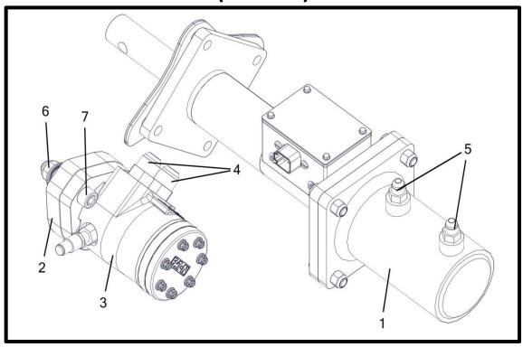
One Section Slide Gate Cylinder & Drive Motor – Tank 1
