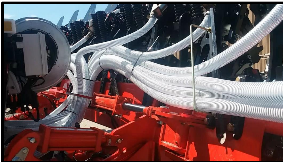
THE HOSES ARE ZIP TIED TOGETHER IN SEVERAL PLACES TO KEEP THEM IN PLACE WHEN THE TOOLBAR FOLDS AND UNFOLDS.
