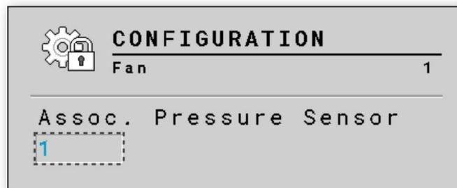
Under the Pressure Sensor, press the selectable area to choose and activate a pressure sensor. Select “1” for main fan.
