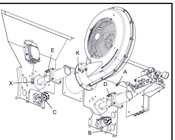
Use this document to install a JD RC2000 controller on a Montag Gen 2 instead of a Montag Dry Rate Controller. This kit is needed to add Slidegate functionality because the RC2000 does not have this function integrated into it. Connect correct harnesses to location on machine indicated by alpha identification. This kit requires Gen 2 to have digital slide gates (shown).
