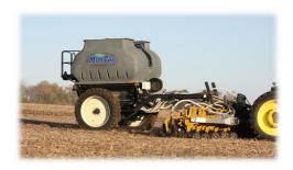
GEN 2 Base Unit with gray bins on a Montag Auto-Steer Cart shown above. Other color options include white and yellow. Bins have two fill inlets each and are independently scaled. All units use the Montag particulate metering system. Multiple U.S. and international patents cover either, or both, this Product and its components.
