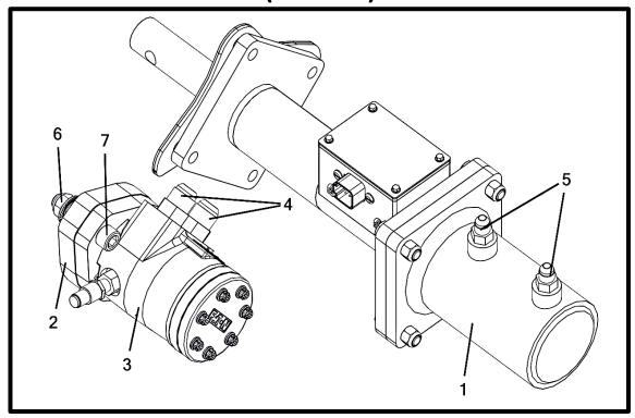
One Section Slide Gate Cylinder & Drive Motor – Tank 1 (Fan End)
