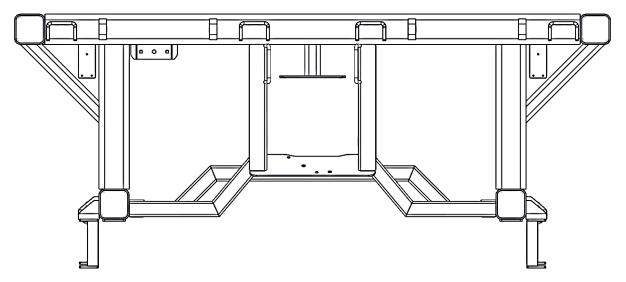
NOTE: BECAUSE OF STS DESIGN, LEGS ON FAN END SIT .5" LOWER THAN THE NON-FAN END
