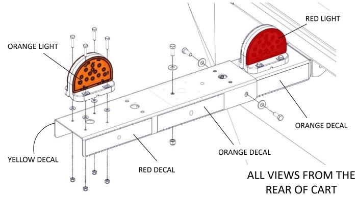
For C12BA (24.5x32" tires) w/160" C/C wheelbase. Install as shown. Note different bracket position in this configuration.
