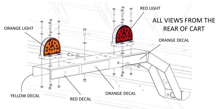
For C12BA (24.5x32" tires) w/160" C/C wheelbase. Install as shown. Note different bracket position in this configuration.
