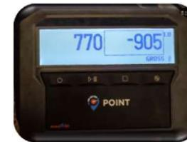
IN ORDER TO CONFIGURE IT, SCALE-TEC NEEDS TO ASSIGN THE MONTAG2 PROFILE TO YOUR DEVICE ONLINE PLEASE PRESS AND HOLD THE 2<sup>ND</sup> AND 4<sup>TH</sup> BUTTONS AT THE SAME TIME. THIS WILL DISPLAY THE SERIAL # WHICH SCALE-TEC WILL NEED.
