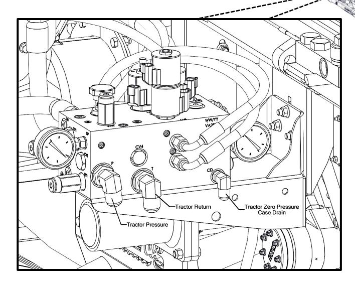
Install hoses in A000177 from tractor to corresponding ports shown.
