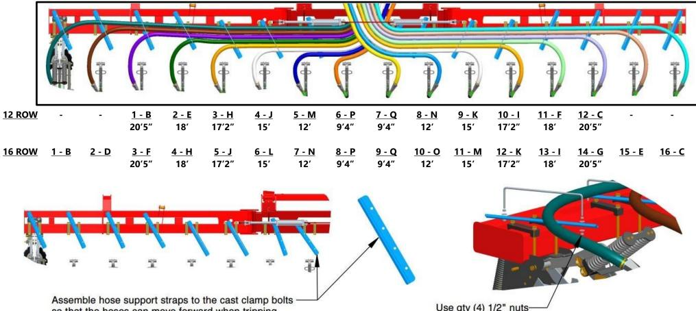
so that the hoses can move forward when tripping over a rock. The center hose supports need to be extended farther back than the wings. Use qty (4) 1/2" nutsand flat washers to mount U-bolts
