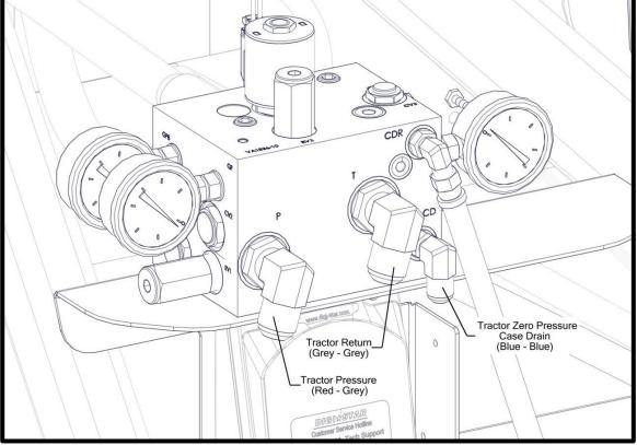
Install hoses in A000109/A000177 from tractor to corresponding ports shown:
