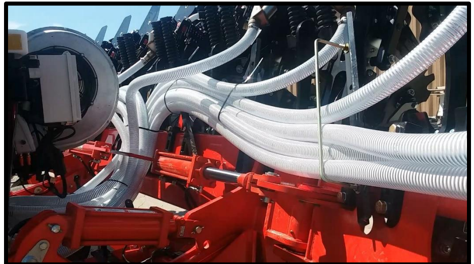
THE HOSES ARE ZIP TIED TOGETHER IN SEVERAL PLACES TO KEEP THEM IN PLACE WHEN THE TOOLBAR FOLDS AND UNFOLDS. SEE THE NEXT PAGE FOR MORE DETAIL.
